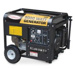
Dual start system: electric and recoil Deliver 9,000W surge, 7,000W continuous 15HP engine Portable system with 10" wheels and handle Outlets: -Three 120V -One 120V/240V -One 12V DC
