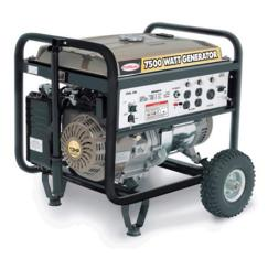
With EPA approval Dual start system electric and recoil Deliver 7,500W surge, 6,000W continuous 13HP engine New AVR system Portable system with 10" wheels and handle Outlets: -Four 120V -One 120V/240V -One 12V DC at 8.3A
