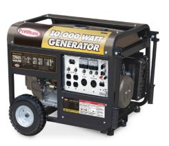
With EPA approval. Dual start system: electric and recoil. Deliver 10,000W surge, 8,000W continuous. 15HP engine with oil alert. Amp and Voltage meters. Fuel gauge. Portable system with 10" wheels and handle. Outlets: -Four 120V 20A -One 120V 30A -One 120V/240V 30A -One 12V DC
