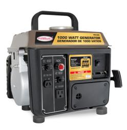
With EPA approval. Recoil Start Deliver 1000W surge, 800W continuous 2HP engine with oil alert Amp and Voltage meters Fuel gauge Portable system with 10" wheels and handle Outlets: -One 120V AC -One 12V DC Master Box: 1 pcs W: 16.70 D: 13.80 H: 14.25 (in) Weight: 44.00 lb / Container 40 STD: 960 pcs Pallet Ti-Hi: 9 Ti / 6 Hi Master boxes per pallet: 54 pcs UPC: 715688073856
