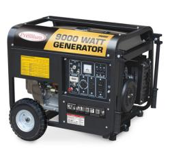
With EPA approval Dual start system: electric and recoil Deliver 9,000W surge, 7,000W continuous 15HP engine Portable system with 10" wheels and handle Outlets: -Three 120V -One 120V/240V -One 12V DC
