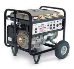
Dual start system electric and recoil Deliver 7,500W surge, 6,000W continuous 13HP engine New AVR system Portable system with 10" wheels and handle Outlets: -Four 120V -One 120V/240V -One 12V DC at 8.3A Master Box: 1 pcs W: 31.70 D: 21.30 H: 23.00 (in) Weight: 195.00 lb / Container 40 STD: 212 pcs UPC: 715688073788
