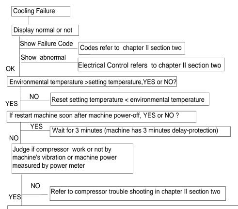
After compressor works, evaporator surface temperature don't go down,the reasons may be the following :
