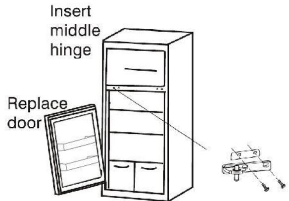
Place the refrigerator door on the bottom hinge. Ensure the door is aligned horizontally and vertically. Attach middle hinge to refrigerator door and attach bolt washer to the back of the hinge, then fix them to middle beam and get them fastened with a screwdriver.
