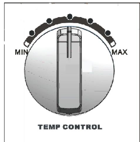
When using the refrigerator-freezer for the first time or after defrosting, turn the temperature control to set "MAX" for at least two hours before introducing the food to be stored.
