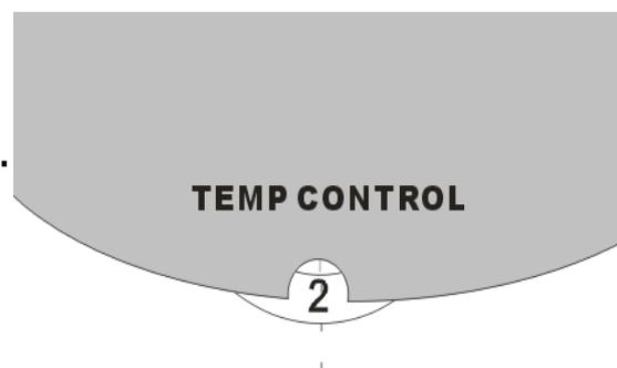
Turn the thermostat control knob up or down to regulate the temperature inside the refrigerator-freezer. The markings on control knob indicated the "1~7" for the different temperature grades. The temperature decreases with position "1" being the warmest and position "7" being the coldest.
